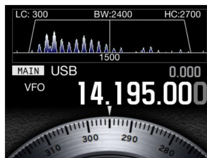
The Sub Scope with Waveform displayed
