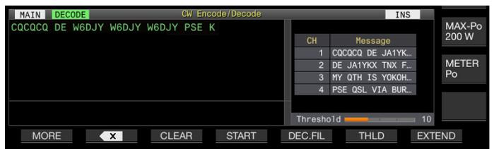
Encoding (Analyzes and Displays the Transmission Code)
