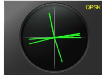
Tuned Correctly (QPSK Mode)
