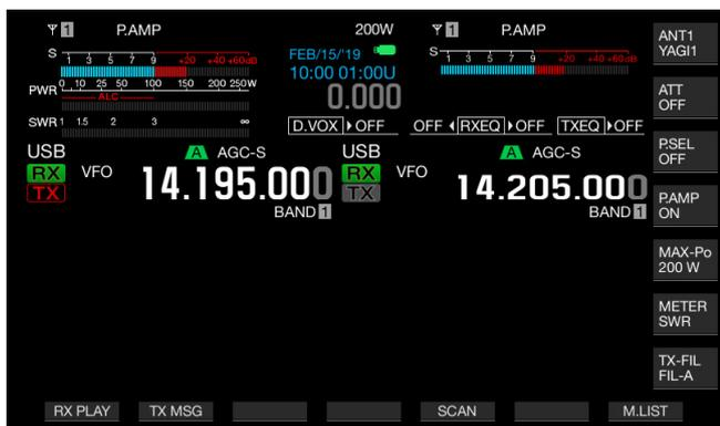
S-meter for the sub band appears on the upper right side of the main display.
